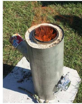
Figure 7: Example Rocket Stove
